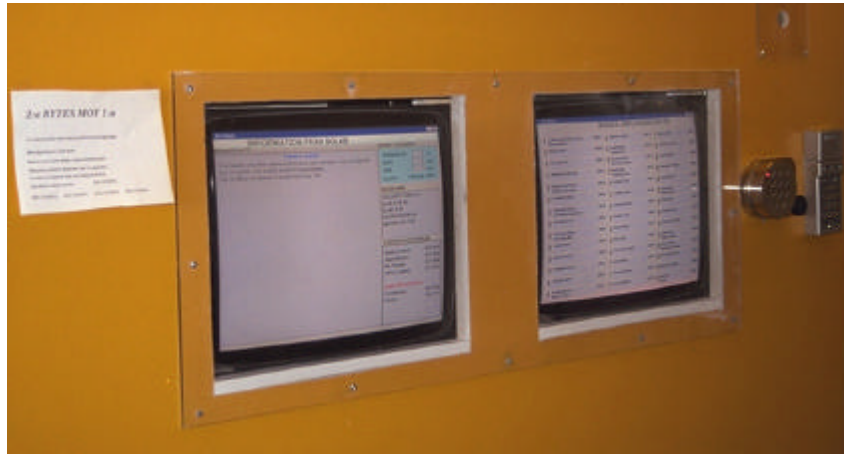
Figure 11. The bulletin board is the screen to the left. On the right hand side there is a screen listing the tenants and their internal telephone numbers (not included in the evaluation of the bulletin board). On the very right one can find the digital key reader, the entrance telephone and a hole for future implementation of a digital videocamera. On the left somebody has left a message on a paper announcing the disappearance of a cat!
