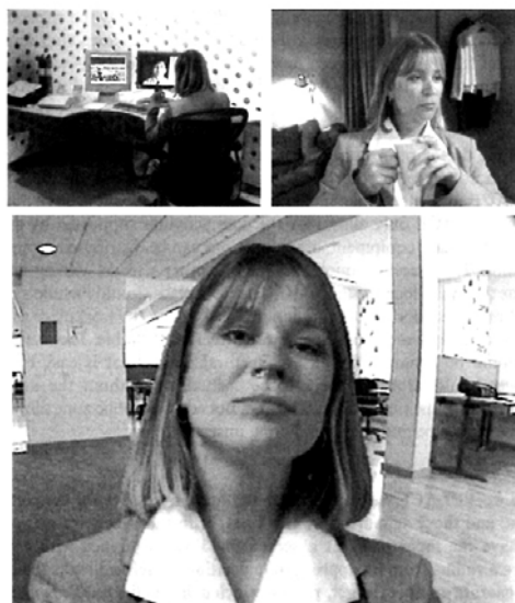
Upper left and right: the user appears as in the real home environment using the videoconference system. Lower image: from the remote place (the perceived image by the partner in the conversation) the user appears to be in an office environment, a process handled by software manipulation of the video image.
