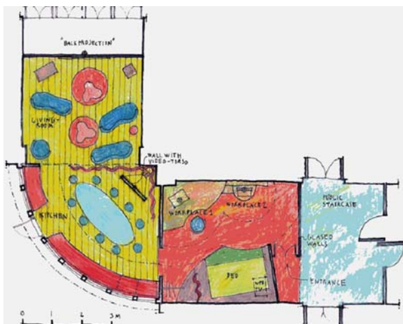
Figure 23. Floor plan sketch of the comHOME flat. To the upper left is the living room. The room at the lower left is the kitchen. The middle room at the bottom is a combined telework and bedroom. At the lower right is the entrance of the buildings public staircase, which does not form part of the flat. (Source: Junestrand & Tollmar, 1999, Paper 2)
